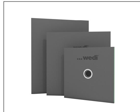
Fundo Solido is installed beneath the PVC covering and takes over the sealing function. An additional surface waterproofing layer is not required. The dry installation method and integrated slope eliminate the need for complex screed work and long drying times.
