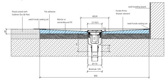
1 The shower element Fundo Nautilo has a thickness of 50 mm.
