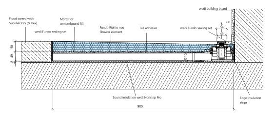
wedi Fundo channel drain vertical, DN 50, screed floor
