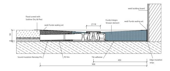
Fundo Integro, complete system A, connection on the long side
