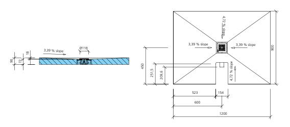
Fundo Integro, complete system B, connection on the short side
