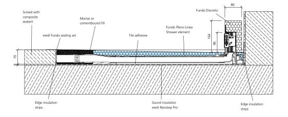
$<sup>^{\</sup>star}$  When using the sound insulation mat, the construction height is increases by 8 or 17 mm.
