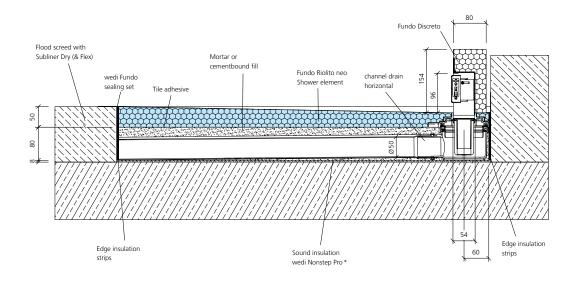
Fundo Discreto, wall drain, DN 40, screed floor
