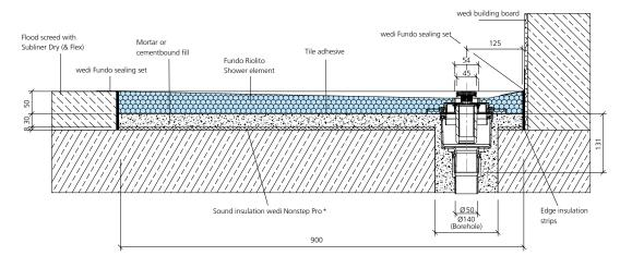
$<sup>^{\</sup>star}$  When using the sound insulation mat, the construction height is increases by 8 or 17 mm.
