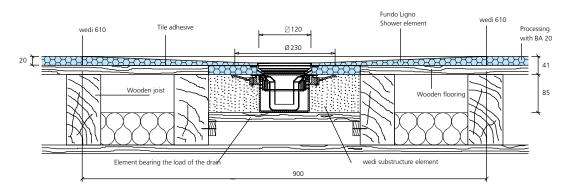
wedi Fundo point drain Mini Max, DN 40, on timber floor
