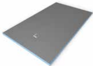
01 wedi Fundo Primo® The original wedi Fundo: Robust, pre sloped, waterproof, shower floor bases with 4" x 4" drain cover. Customizable on site. Often installed on substrates and used with wedi curbs.
