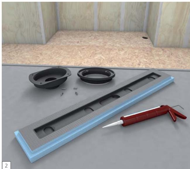
**EN** Assemble the drain unit following the instruction drawing. wedi's Riolito neo bases can be cut to size on all sides making drain positions close to the wall possible. Please do not cut into the linear drains plastic flange integrated into the coated foam part of the base. Once cut the 1/2" x 1/2" channels at the new base perimeter must be reestablished. When cutting close to the drain channel always leave enough wedi foam for re-making the needed 1/2" x 1/2" channel.
