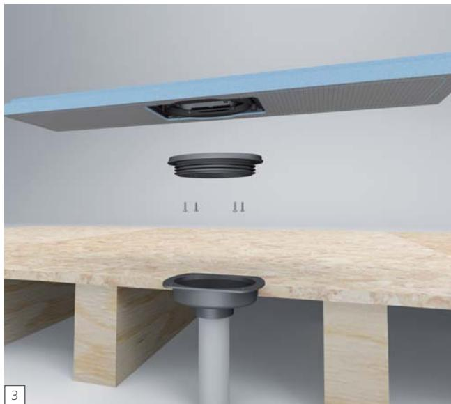
**EN** Glue and seal the wedi drain trap to the 2" pipe using appropriate solvent cement glue for the plastics involved. Do not screw drain body/trap to floor. Secure with some dabs of wedi joint sealant under flange instead. Mount the oval sealing collar/ gasket to the base's receiving ABS plastic channel on it's underside with no gaps showing in between both parts. Use only the wedi screws provided and manually tighten with a phillips screwdriver.
