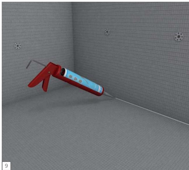
**EN** Apply continuous 1/2" (13 mm) bead of sealant between all connections of panels and install with tightly butted seams. Excess sealant must be spread flat with a putty knife. All seams and fastener heads in the assembly are covered with a secondary 1/2" (13 mm) bead of sealant and spread flat. The seams should be covered 3/4" to 1" (19 mm to 25 mm) on either side of seam. All fastener/washers are covered with sealant stretching 1" (25 mm) over the washer edges.
