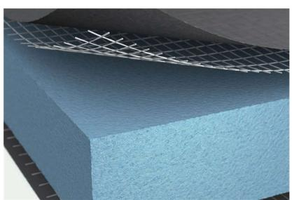
With wedi building boards, bathrooms can be effectively and easily insulated from the inside. The thermally insulating board with XPS core is waterproof and provides an optimal base for tiles and other floor, wall and ceiling coverings. Depending on the external wall, the heat loss can be reduced by more than half with just 20 mm thick wedi building boards.
