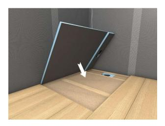
Owing to its low installation height of just 25 mm, the Fundo RioLigno shower element can be integrated perfectly flush with existing floorboards.
