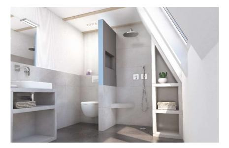
In the wedi Sanwell element, the niche is already integrated in the factory. Complex sealing, as in brick walls, is no longer necessary.
