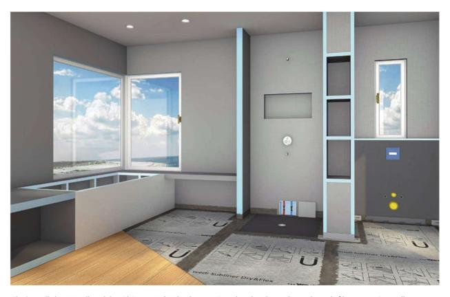
The Sanwell shower wall module with integrated technology was introduced to the market at the end of last year. It is equally suitable for installation on the existing substrate as a fixed wall or as a free-standing shower partition. The special features are the pre-installed cold and hot water pipes as well as the integrated Hansgrohe iBox allowing for more than 200 thermostatic mixer designs.
